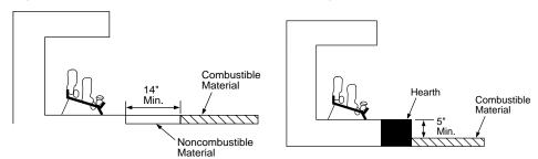
Figure 8 - Minimum Fireplace Clearances If Installed at Floor Level
